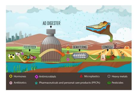
**Figure 17.1** Agricultural farm with an AD digester used for the manure treatment and later used as biofertilizer. The fate of some pollutants flowing during the whole process is shown with different symbols.
