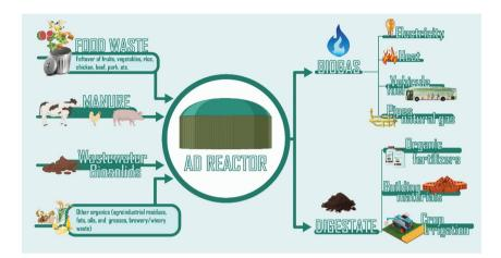
Figure 17.2 Potential inputs and outputs that an AD reactor can manage and different scales.
