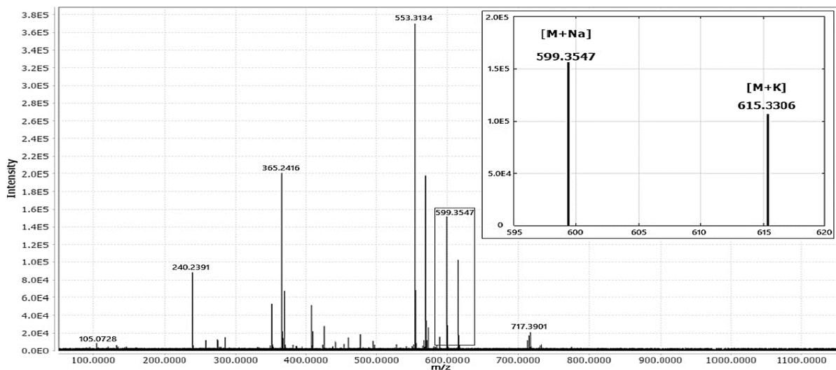
**Figure 9. Oleandrin identification in *cf. A. excelsum* extract by LC-MS analysis. Ions identified: [M+Na]<sup>+</sup> 599.3547 and [M+K]<sup>+</sup> 615.3306 at retention time: 7.52 min.**
