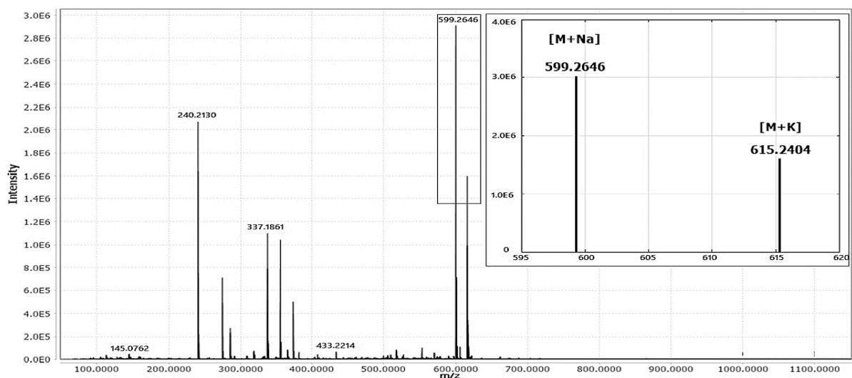
**Figure 8. Oleandrin identification in *H. tarapotensis* extract by LC-MS analysis. Ions identified: [M+Na]<sup>+</sup> 599.2646 and [M+K]<sup>+</sup> 615.2404 at a retention time: 7.52 min.**
