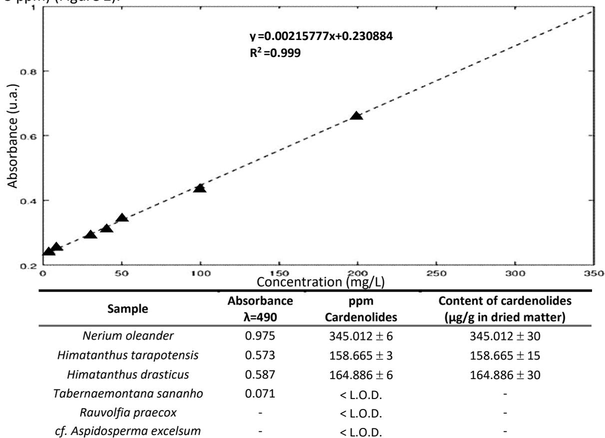
**Figure 2.** Calibration curve with fit linear (First Order) made with oleandrin standard solutions. Determination of total cardenolides similar to oleandrin by UV-Vis-NIR spectrophotometry using Baljet's reagent.
