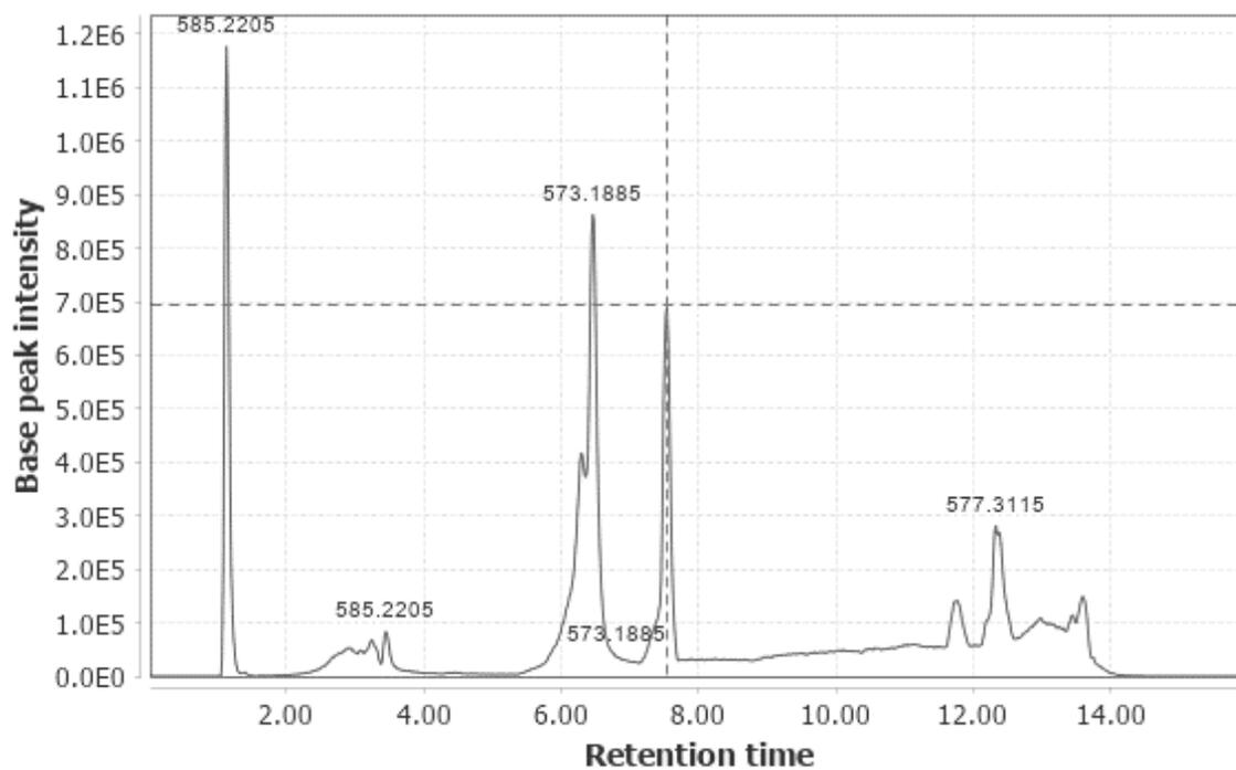
**Figure S1.** LC spectrum from HPLC-QTOF-MS analysis for oleandrin standard at retention time: 7.54 min.
