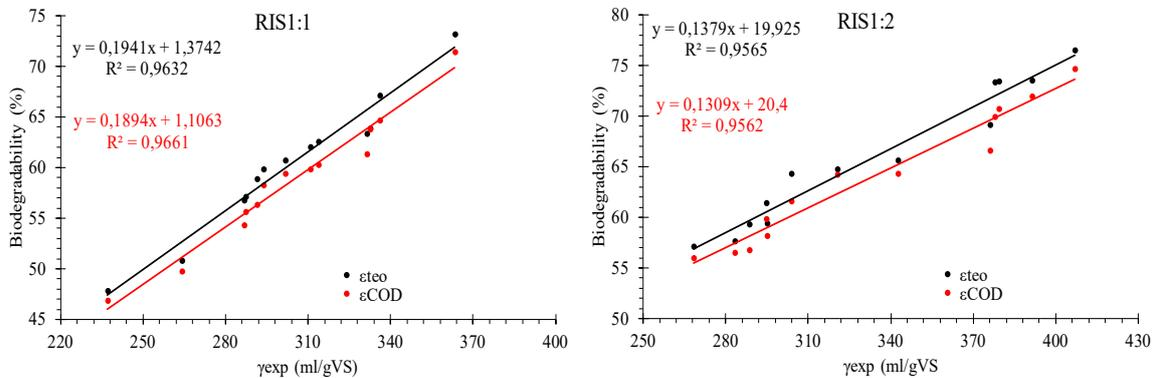
353 Figure 4. Effect of experimental performance  $\gamma_{\text{exp}}$  on biodegradability:  $\epsilon_{\text{teo}}$ : biodegradability based on  $\gamma_{\text{teo}}$ ,
