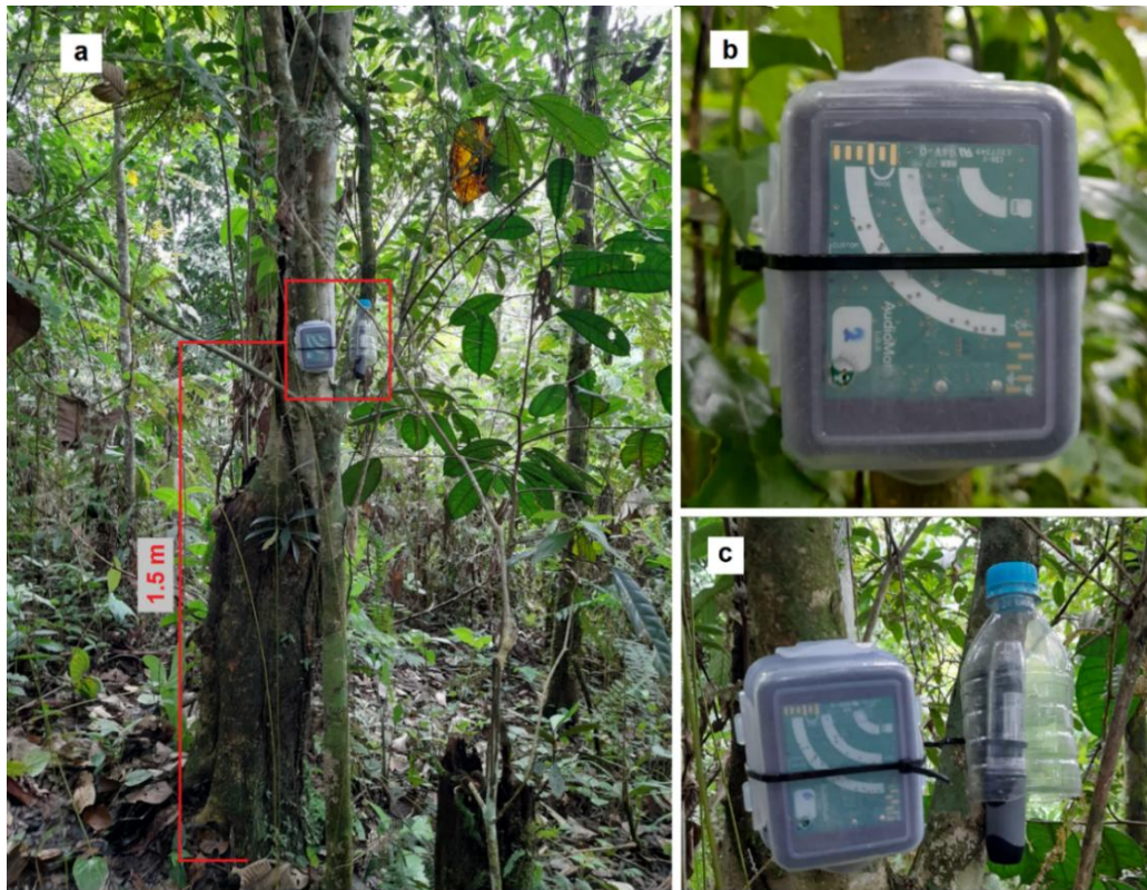
Figure 2. AudioMoth recorders set up: a) Installation of equipment 1.5 m above the ground, b and c) Deployed recorder and datalogger handmade enclosure. Made by: López, 2023.
