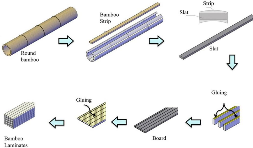
Figure 1. Manufacture of bamboo laminates. Adapted from Figure 1 [32,33].
