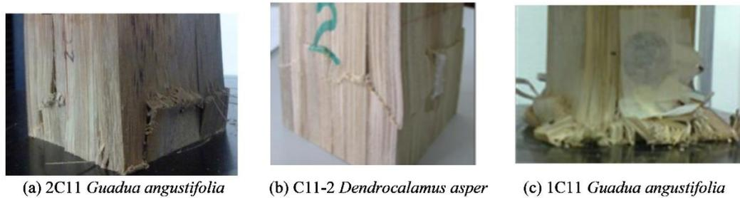
Figure 8. C11 Specimens' failure. Source: Authors
