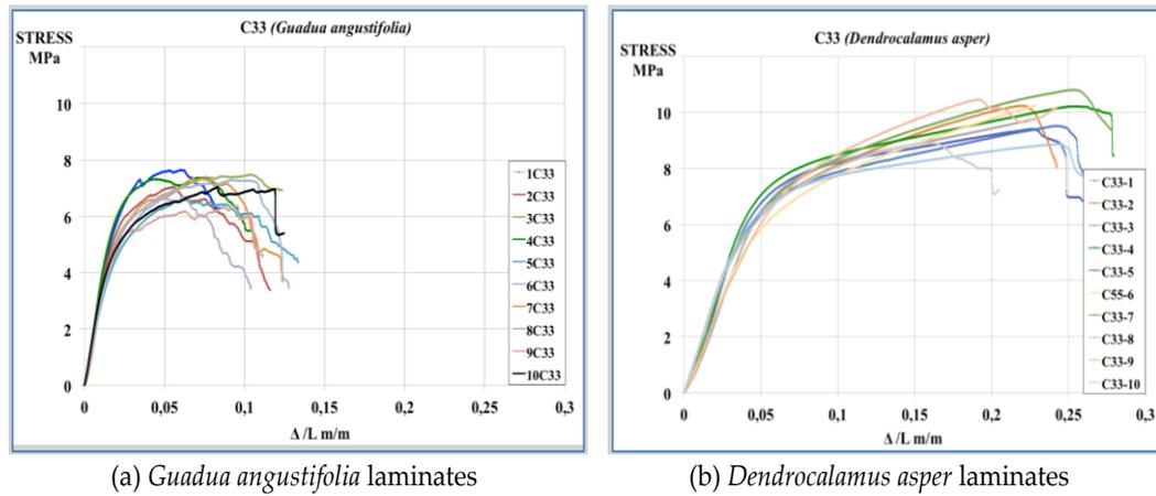
Figure 7. Stress vs  $\Delta/L$  (Compression perpendicular to the fibre and parallel to the boards C33). Source: Authors.
