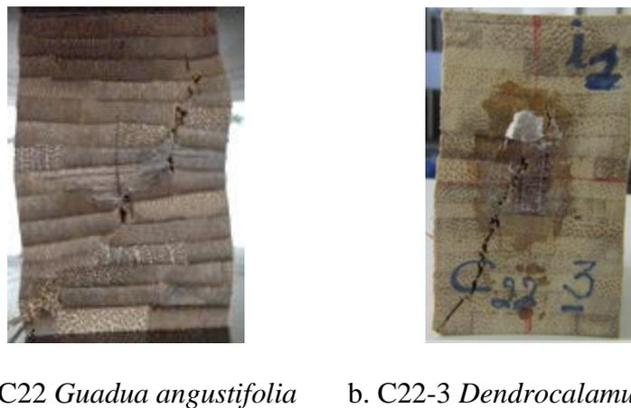
Figure 9. C22 Specimens' failure. Source: Authors
