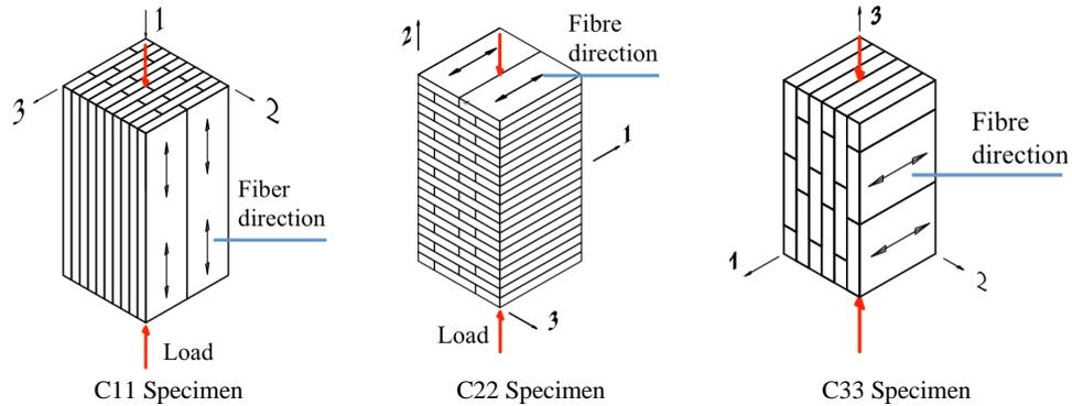
Figure 3. Nomenclature and codes used for specimens. Adapted from Figure 2 [32].
